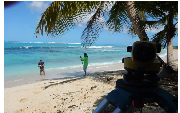
Rich S. and Art. C. laying out the transect during high tide and surf conditions at Tachonga South 1. On the right is the Berger Level on the tripod.
