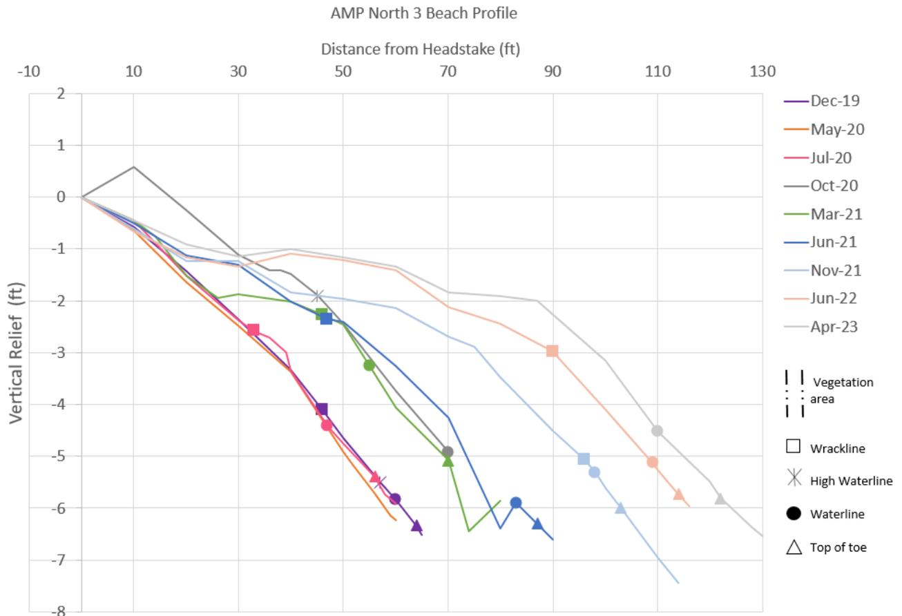
**Figure 6 - Beach profile of AMP North 3 showing profiles from December 2019 - April 2023. The distance from the headstake in feet is shown here with the elevation differences starting from the headstake.**
