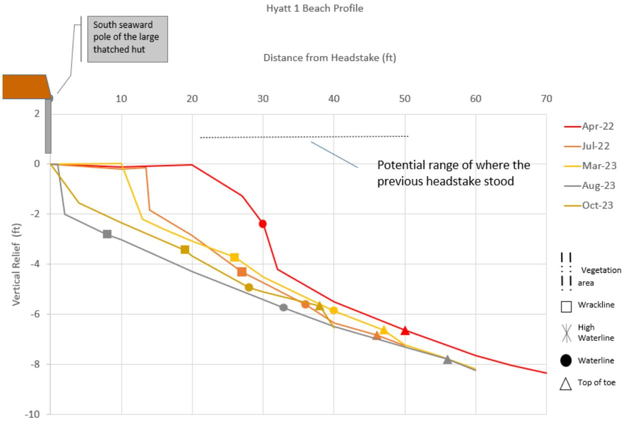
This beach profile illustrates the shoreline's 2D contour by plotting length and relative elevation of a headstake, or a routinely monitored starting point, to past the waterline. This is a data product from the Bureau of Environmental Coastal Quality - Division of Coastal Resources Management (BECQ-DCRM). Contact [planning@dcrm.gov.mp](mailto:planning@dcrm.gov.mp) for any clarifications or questions regarding this data. Award No.: NA22NOS4190158
