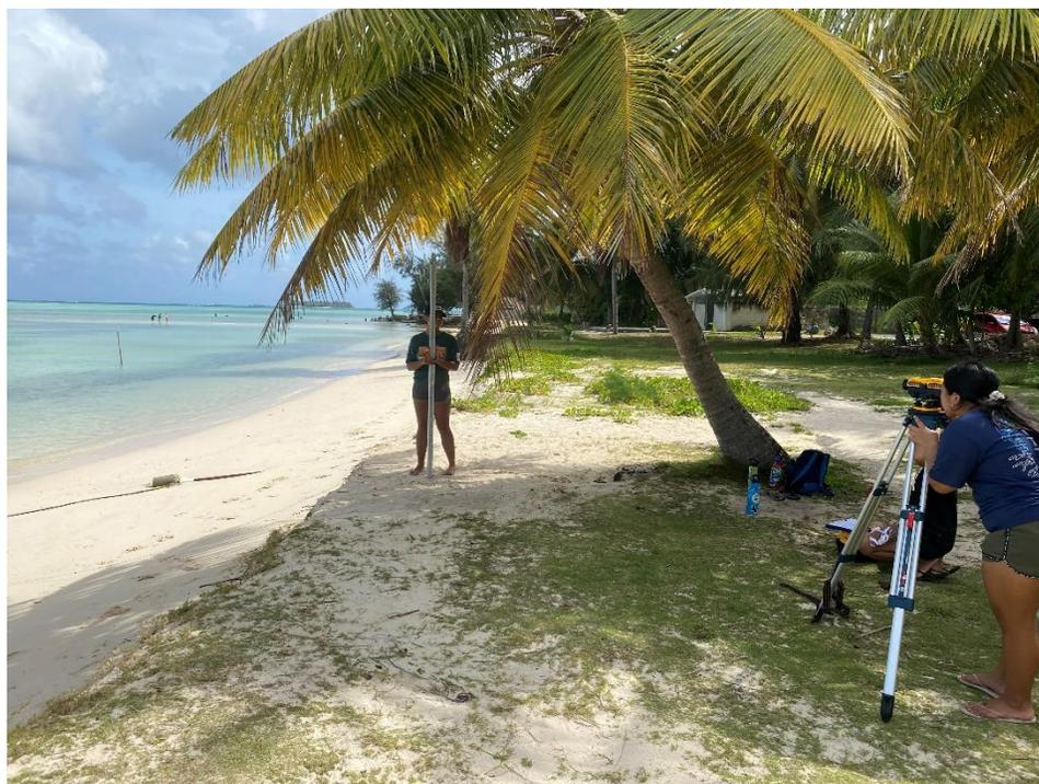
**Figure 1 - At a beach between Crowne Plaza and Hyatt, Kyla looks through the Berger level, an instrument mounted on a tripod. Emma holds a rod level, a measuring instrument for height, along a transect line to capture the eroding beach profile.**
