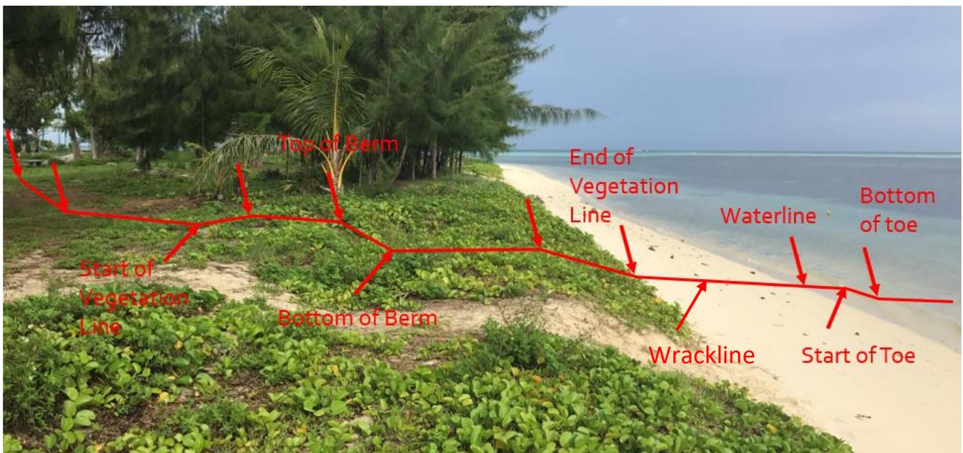
**Figure 5 - The common features of a beach profile noted during surveying.**
