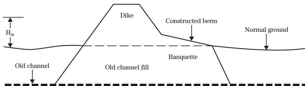
The use of highly permeable soil in the dike should be avoided when possible because of potential leakage and piping. Where highly permeable soil is used in the dike fill, especially over a more slowly permeable foundation, the landside base of the dike may need to be extended, or a toe drain provided to increase the dike's stability. The phreatic line should be contained within the embankment cross section. The additional width or drainage may be provided in the manner shown in figure 13-14.
